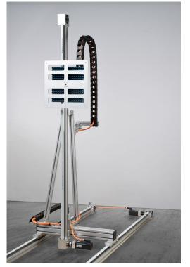
5G Antenna Positioning System for 5G Sub 6 GHz OTA Chamber
