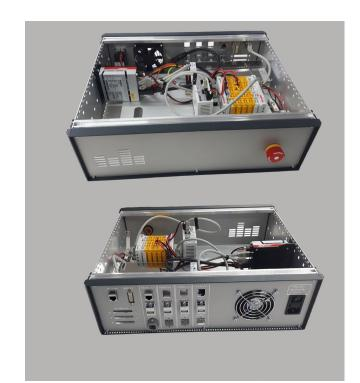
Controller for Antenna & DUT Positioners
